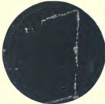
Fig. 16. White native silver filling cleavage cracks in dark calcite. This structure terminates an irregular, much thicker vein, the end of which is seen at the lower right-hand corner.
